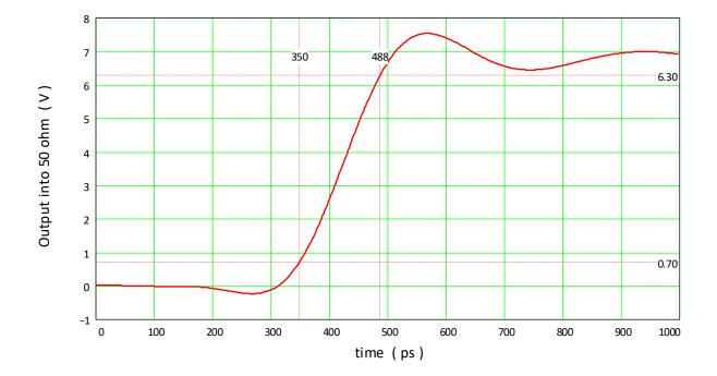
Typical signal outputs from the CAL-07 unit measured using a 3 GHz bandwidth digital sampling oscilloscope with a sampling rate of 10 GSa/s, using  $\sin(x)/x$  interpolation:
