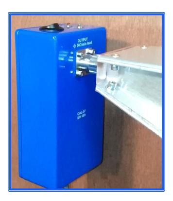
CAL-07 unit attached to the input of a UHF GTEM calibration system
